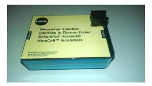
Connect the standard Cat5 cable from the top-mounted RJ45-jack on the interface labeled "NTMS" to one of the NTMS data jacks.
