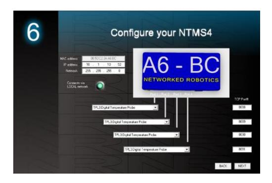
4. Click on the drop-down for the physical port on the NTMS where the probe is connected, and under the "Device Type" drop down, select DCP/LVP/RTD.
